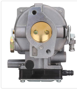
Front view of the carburetor, showing the air intake opening.
