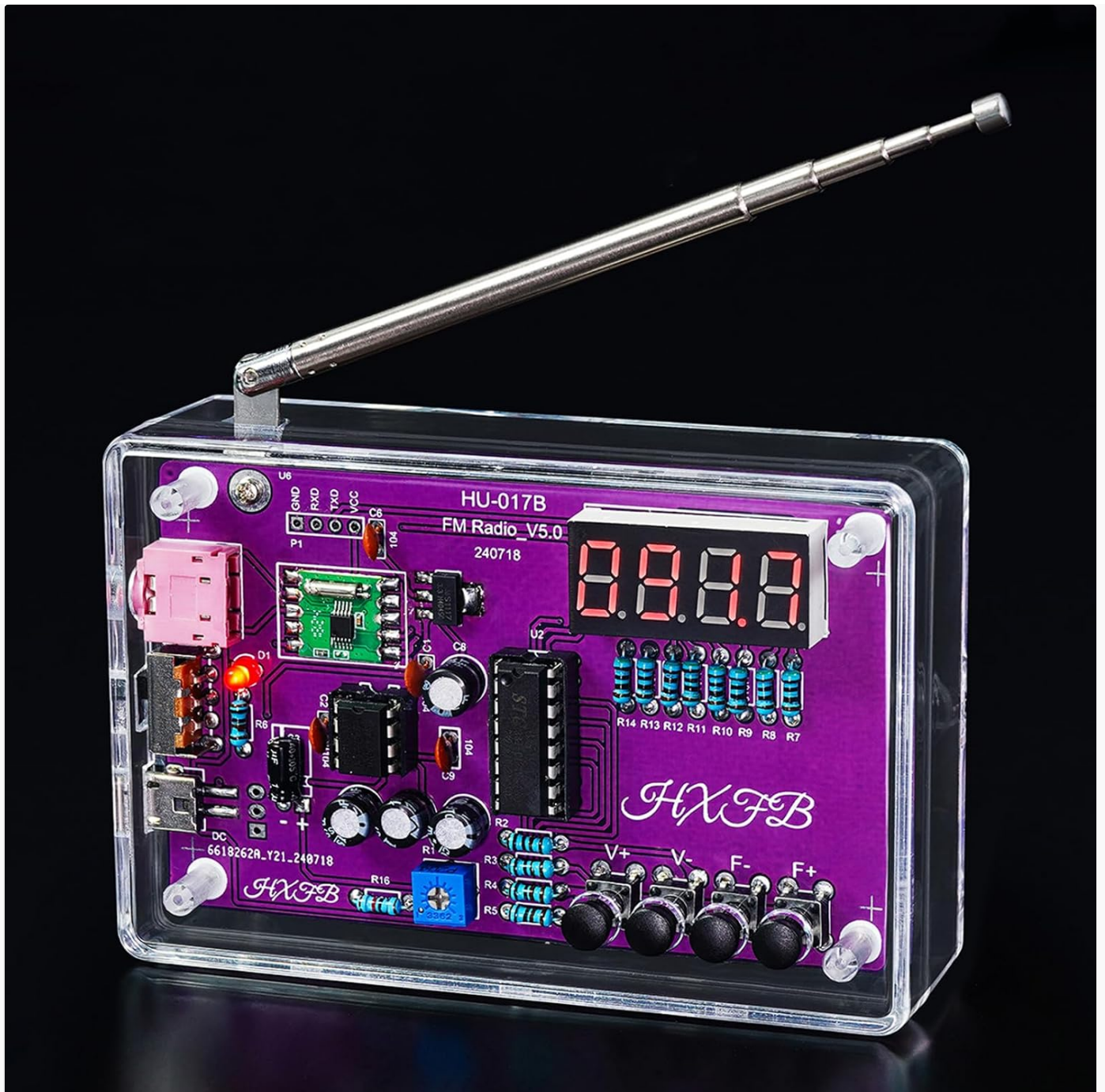
Image: The fully assembled RDA5807 FM Radio, showcasing its clear acrylic casing, purple PCB, digital display, and telescopic antenna.
