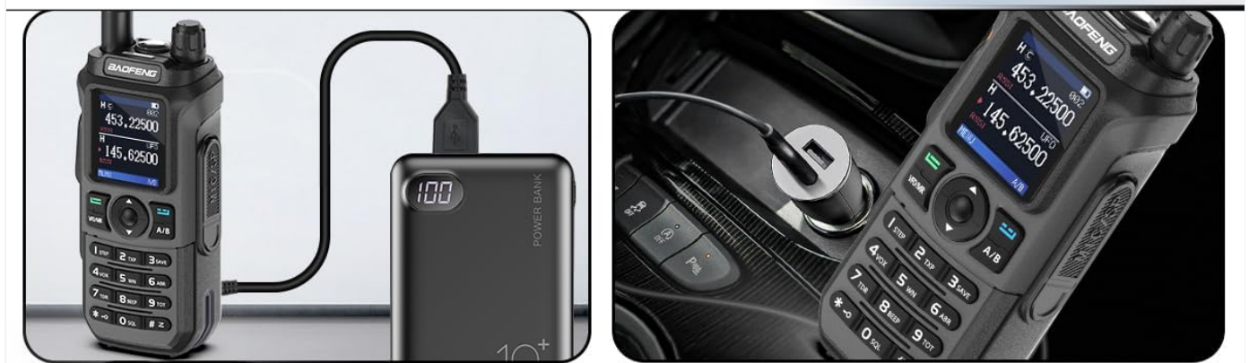
Figure 2.1: The BAOFENG UV-21R supports both Type-C USB charging and traditional base charging.
