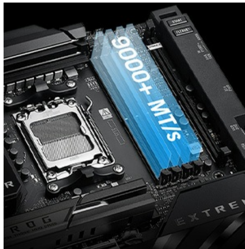
Image: Illustration showing DDR5 memory modules installed in the motherboard slots.
