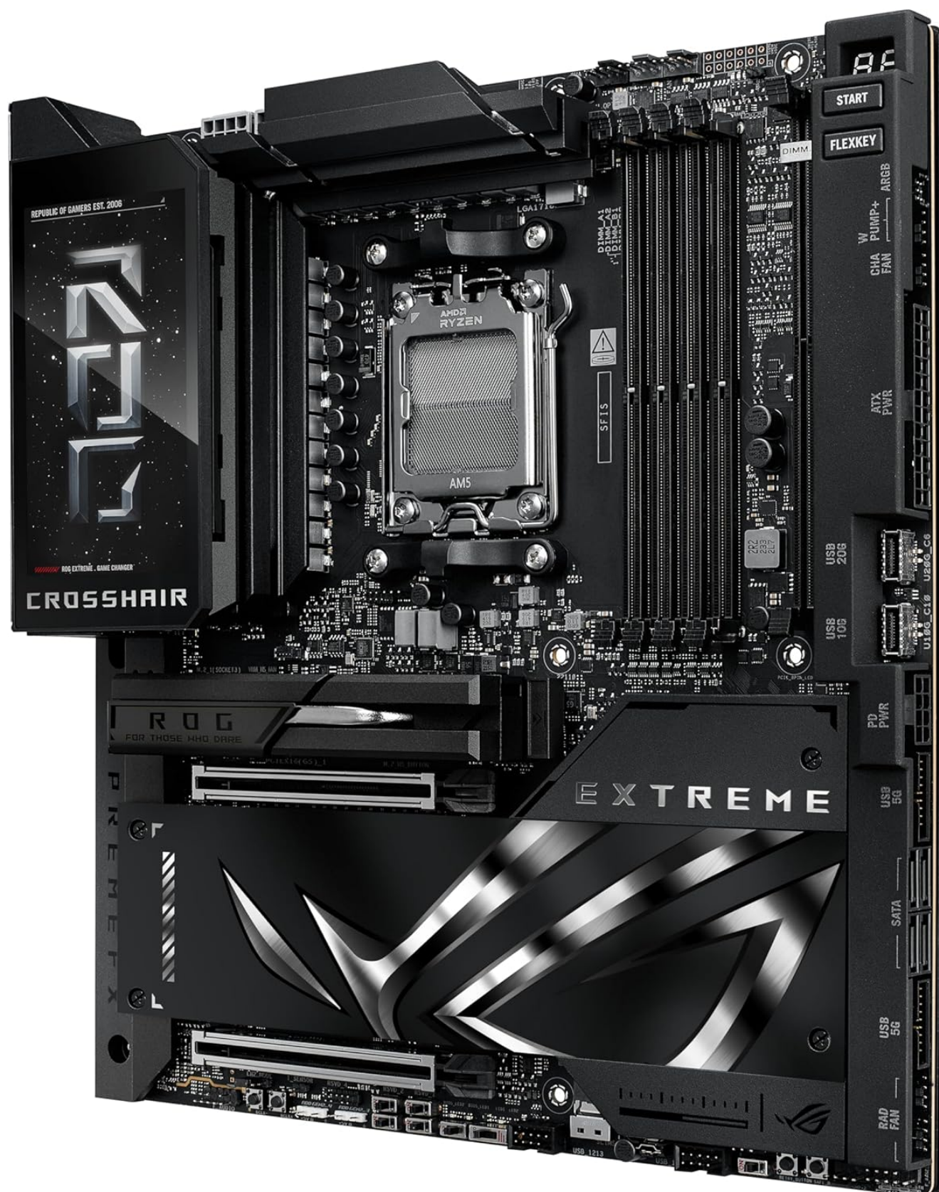
Image: Angled view of the motherboard, focusing on the AM5 CPU socket.
