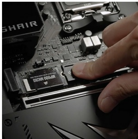
Image: Demonstration of the M.2 Q-Latch for tool-less SSD installation.
