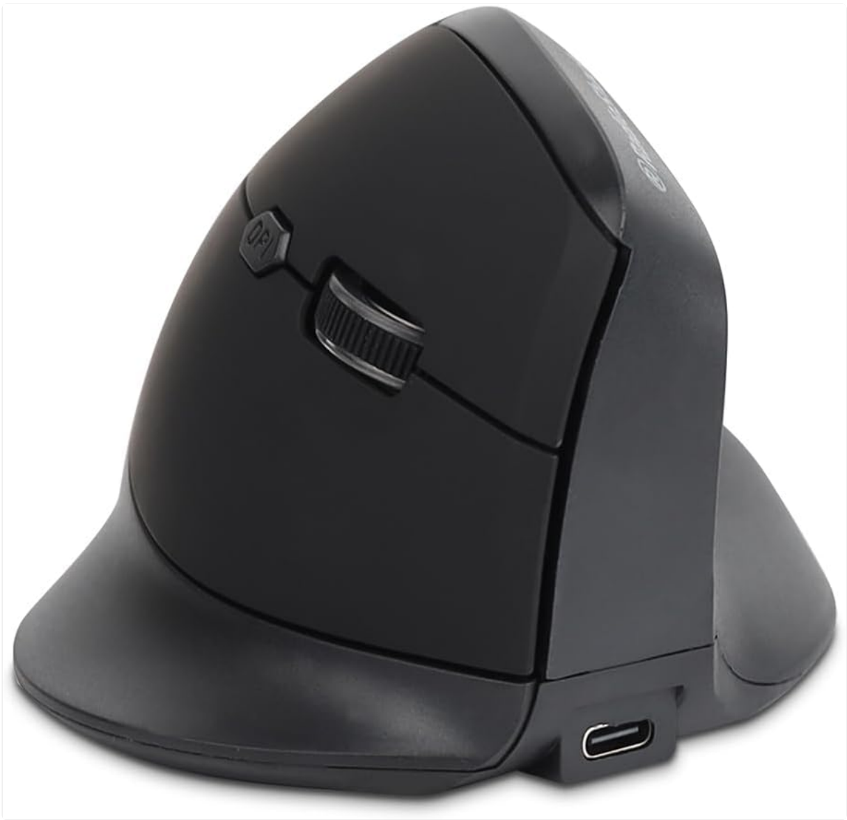
Figure 3: Side view of the mouse highlighting the USB Type-C charging port.
