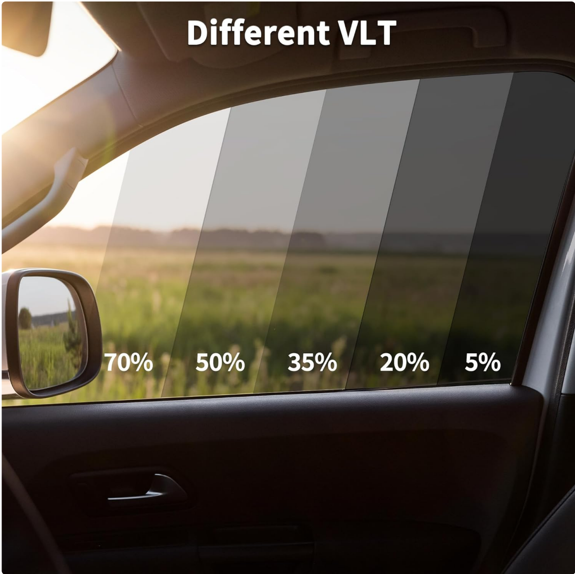
Image 2: Illustration of various Visible Light Transmission (VLT) levels on car windows, demonstrating the visual effect of different tint percentages.
