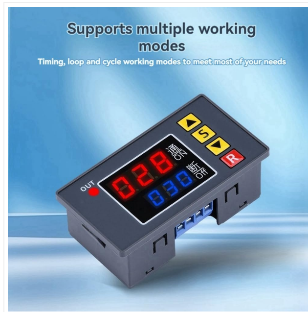
Figure 4.1: The T3231 controller highlighting its capability to support various timing and cycle modes, indicated by the display and control buttons.
