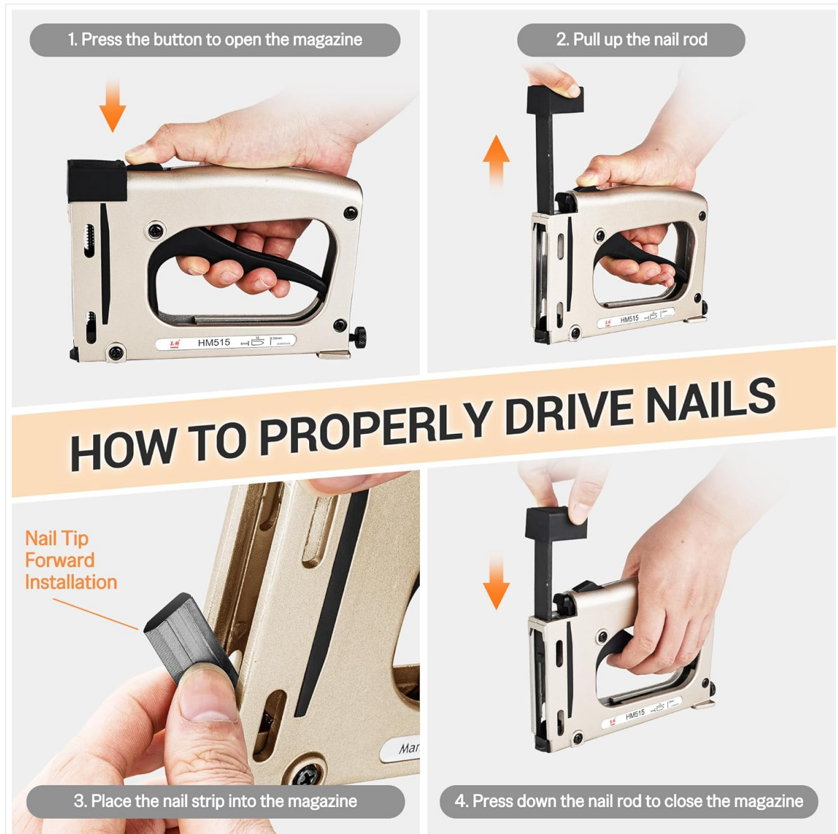
Figure 2: Steps for Loading Flexible Points. This image illustrates the process of opening the magazine, pulling the nail rod, inserting the point strip, and closing the magazine.
