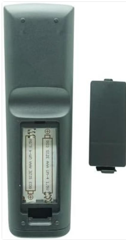
Figure 1: Battery compartment with cover removed, showing slots for two AAA batteries.
