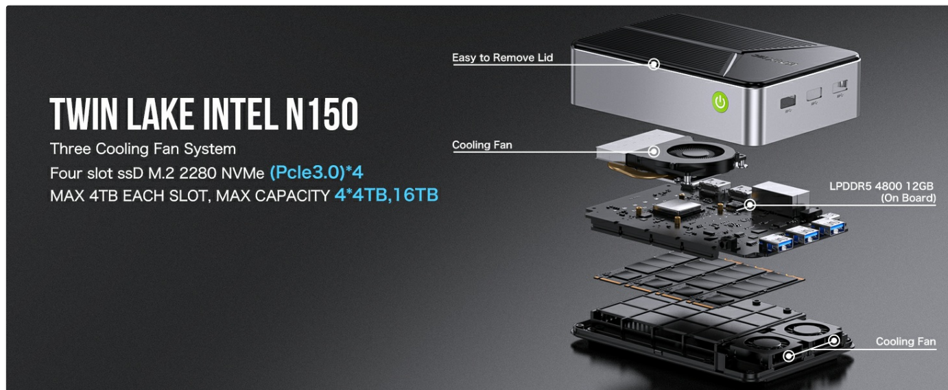
Image 6.2: Exploded view of the GMKtec G9 Mini PC, highlighting its internal components and triple cooling fan system.
