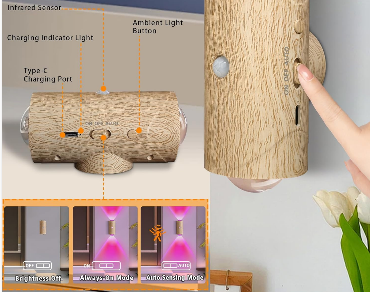
Image: Detailed view of the night light, highlighting the infrared sensor, charging indicator light, Type-C charging port, ambient light button, and the ON-OFF-AUTO switch.
