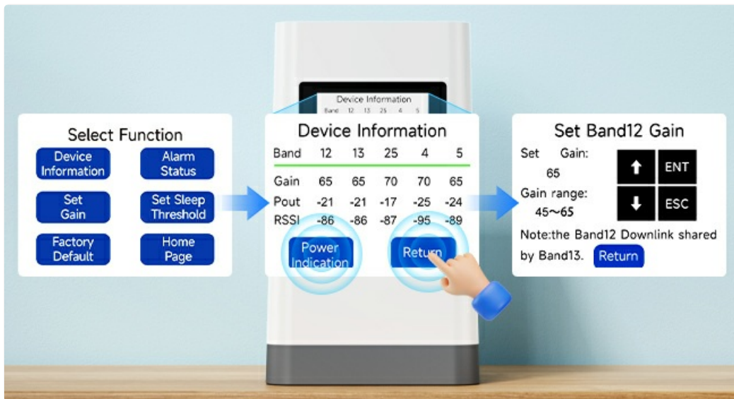
Figure 5.2: The F40-OL's LCD screen interface, showing the "Select Function" menu with options like "Device Information", "Set Gain", "Alarm Status", "Set Sleep Threshold", and "Factory Default". It also illustrates the process of adjusting gain for a specific band, such as Band 12.
