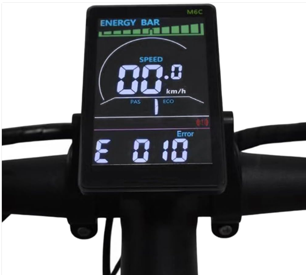
Image: The Wuden M6C LCD Display Meter screen showing an error code 'E 010', indicating a system fault.
