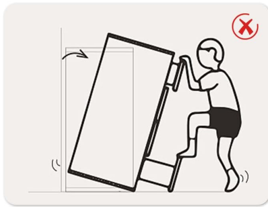
Image 2.1: Illustration of the anti-tip kit and proper installation to prevent tipping, with diagrams of correct and incorrect usage.
