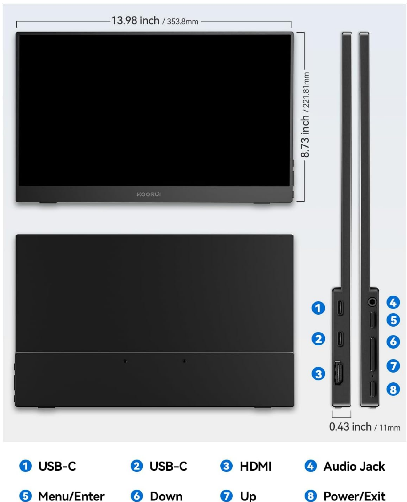
Image 3.2: Monitor Ports and Buttons Layout
