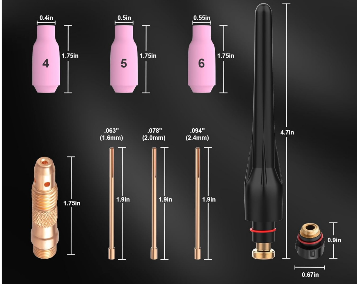
Image: Diagram illustrating the dimensions and sizes of the ceramic cups, collets, collet body, and back caps for the WP-17V TIG torch.
