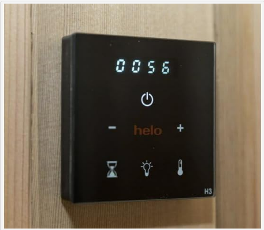
Figure 2.2: The Amerec H3 Control Panel, used for managing sauna settings.
