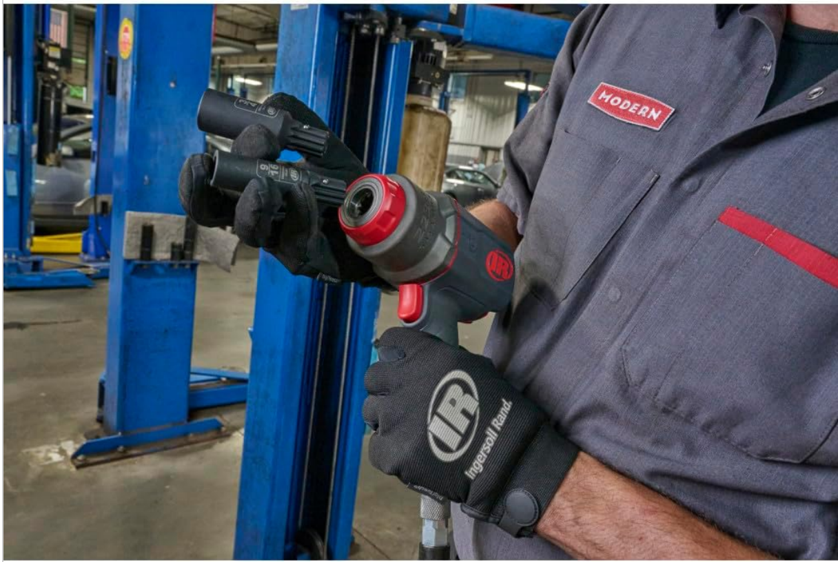
Figure 2: Proper attachment of the DXS2 socket to an Ingersoll Rand impact wrench. The image illustrates a user securing the socket onto the tool's drive.
