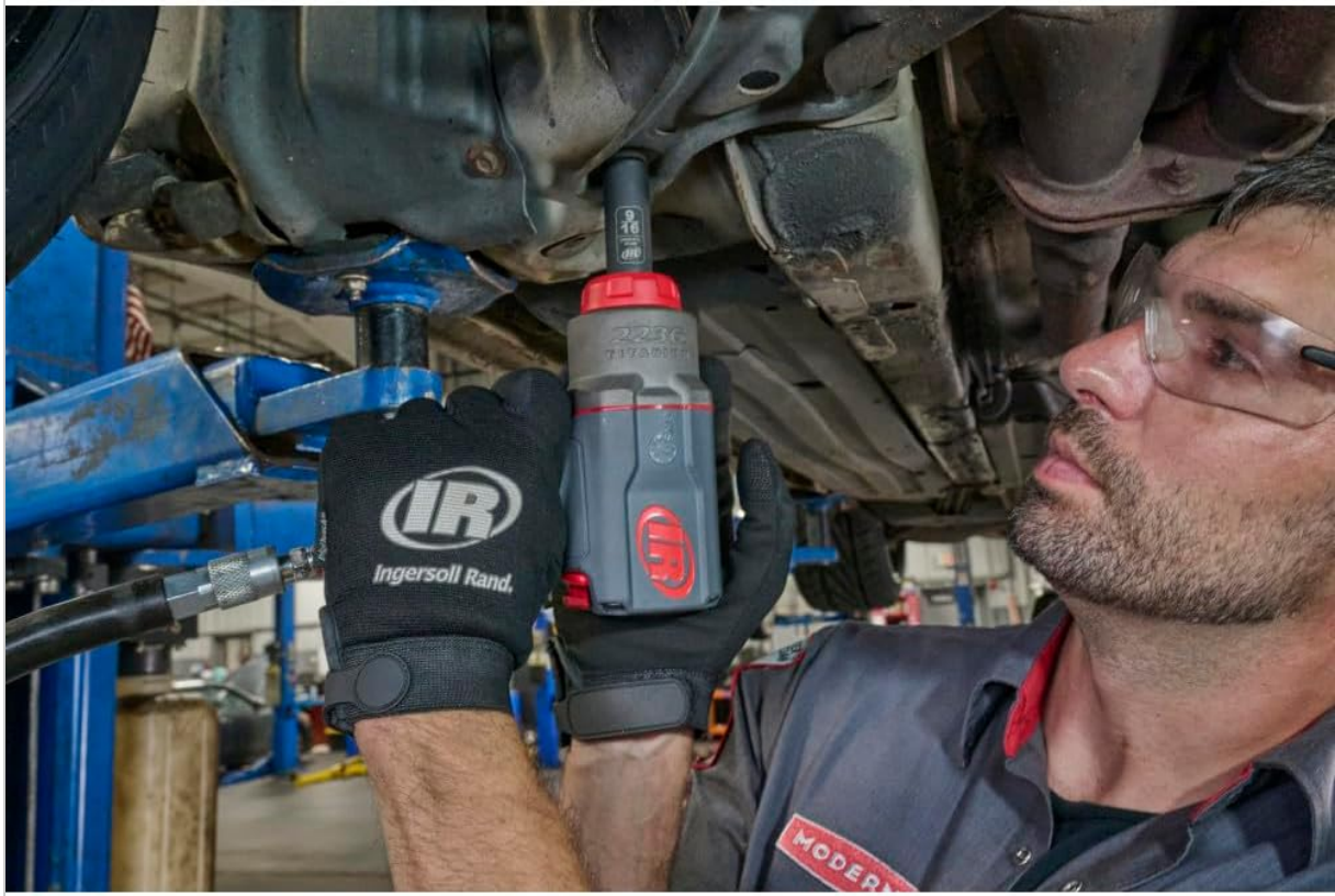
Figure 3: Demonstrating the use of the DXS2 socket with an impact wrench to access a fastener in a restricted area. The image shows a mechanic working under a vehicle.
