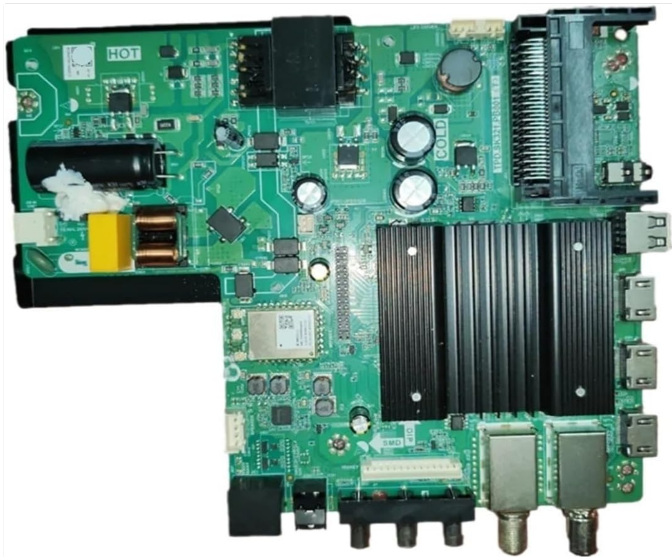
Figure 2: Front view of the TPD.SK321.PB801(T) motherboard, displaying multiple input/output ports (HDMI, USB, antenna) and a prominent heat sink for cooling.
