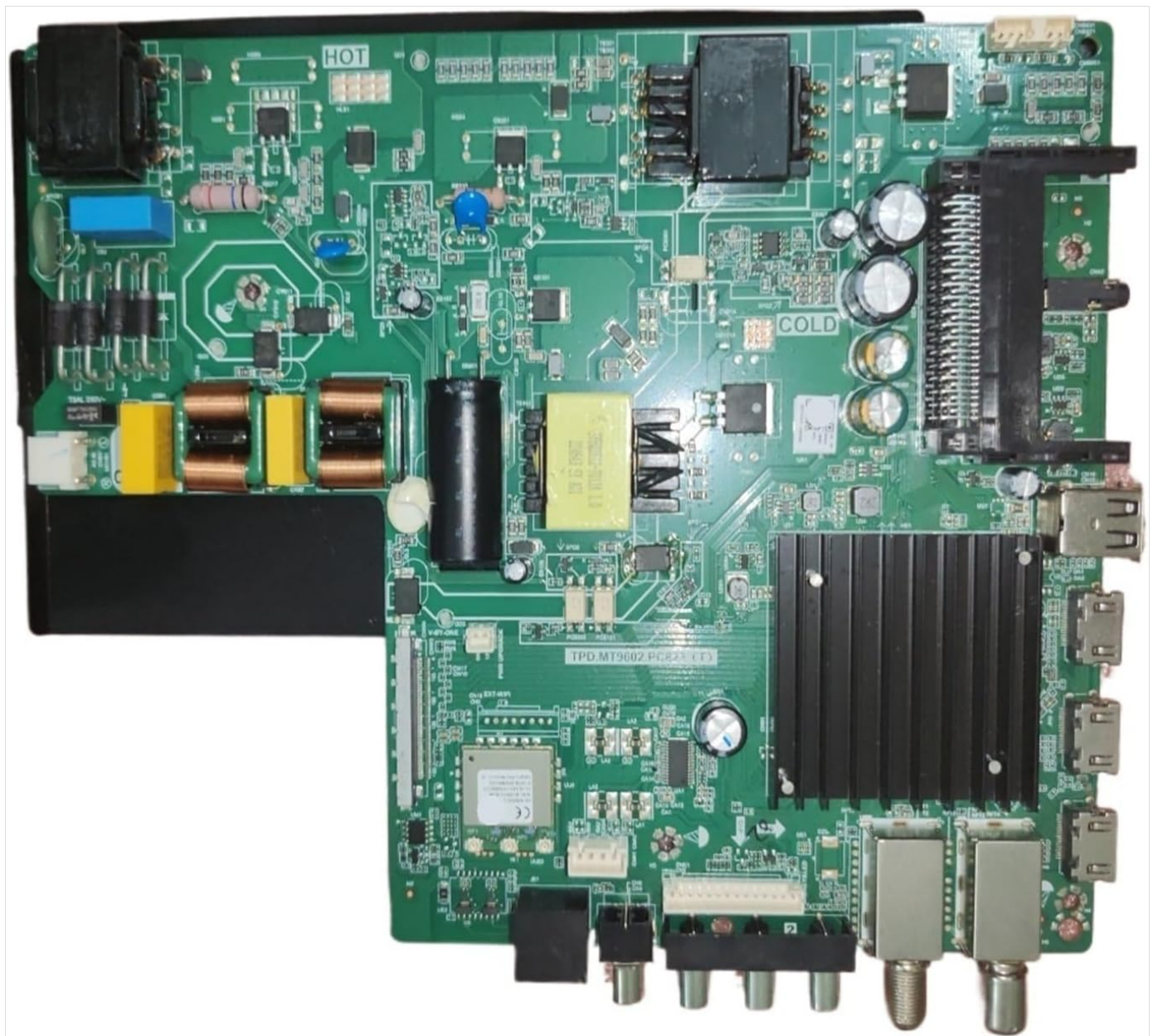
Figure 3.2: Angled view of the RXCWWZQQ TPD.MT9602.PC823(T) 4K TV Motherboard. This perspective provides a clearer look at the connectivity options, including multiple USB ports and HDMI inputs located along the right edge of the board, as well as coaxial cable inputs at the bottom right.
