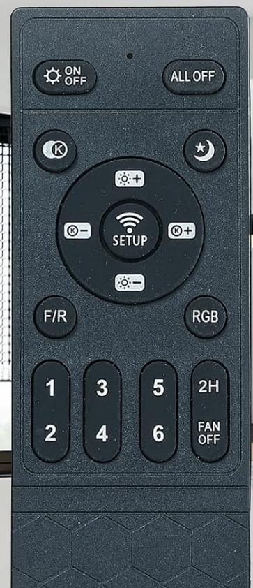
Figure 4: Remote control layout with functions for fan speed, light color temperature (3000K-6500K), timer, and forward/reversal modes.
