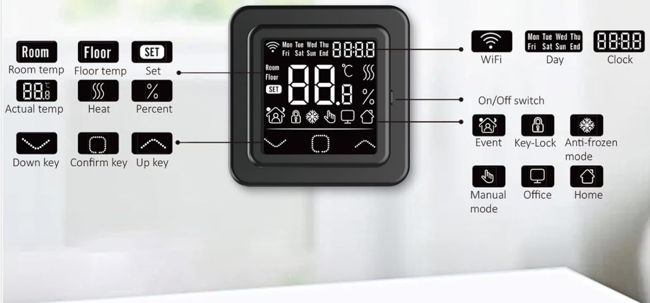
Image 4.1: Explanation of thermostat symbols, including buttons for confirmation, parameter selection, and icons for WiFi, heating, modes, and sensor types.
