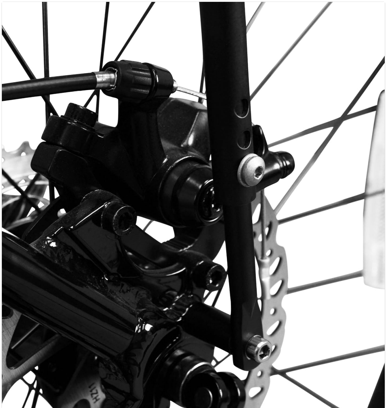
Image: Close-up view of the lower mounting arm installation, demonstrating clearance for the disc brake caliper. The rack is designed to accommodate disc brake systems.
