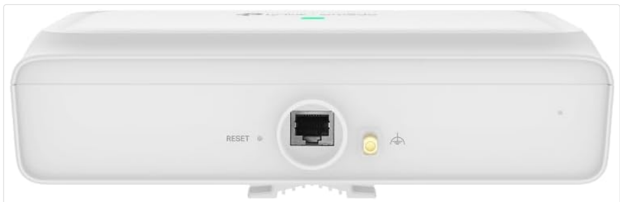
Figure 3.2: Bottom view of the access point, featuring the Reset button, 2.5G Ethernet port (PoE+), and grounding terminal.
