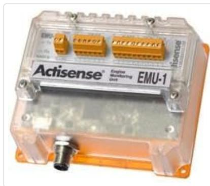
*An image showing the Actisense EMU-1 device with its clear casing, revealing internal components and screw terminal connections.*
