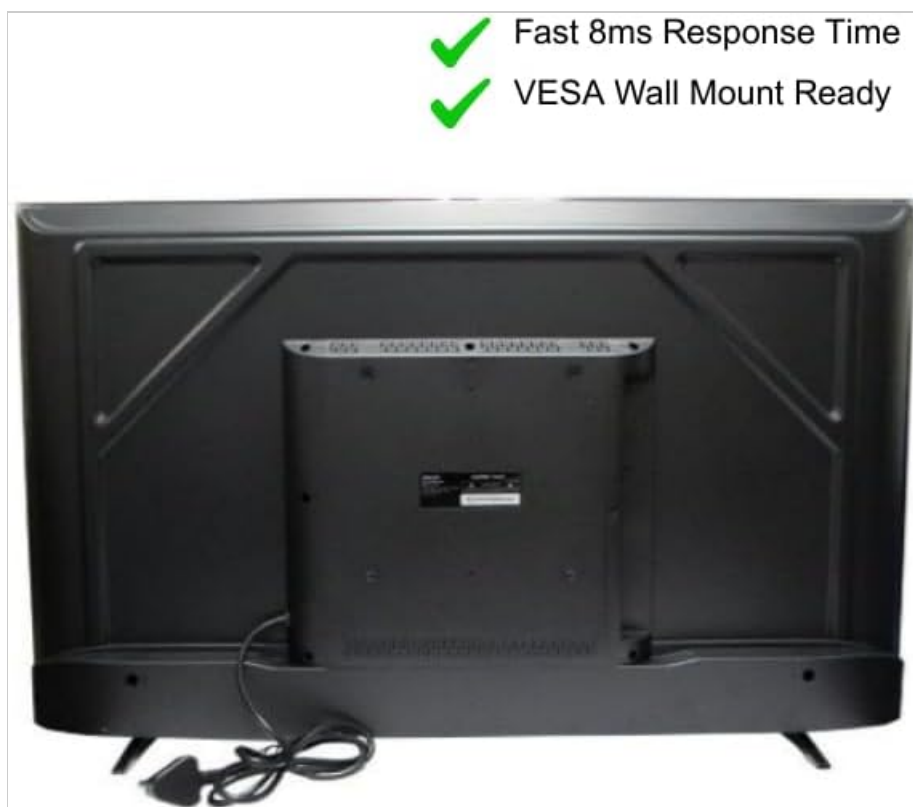
Image: Rear view of the Mecer 43 inch monitor, illustrating the VESA wall mount points and the location of various input ports.
