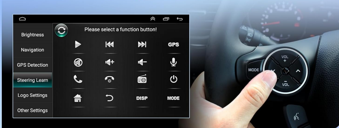
Figure 6: Reverse display and steering wheel control setup.
