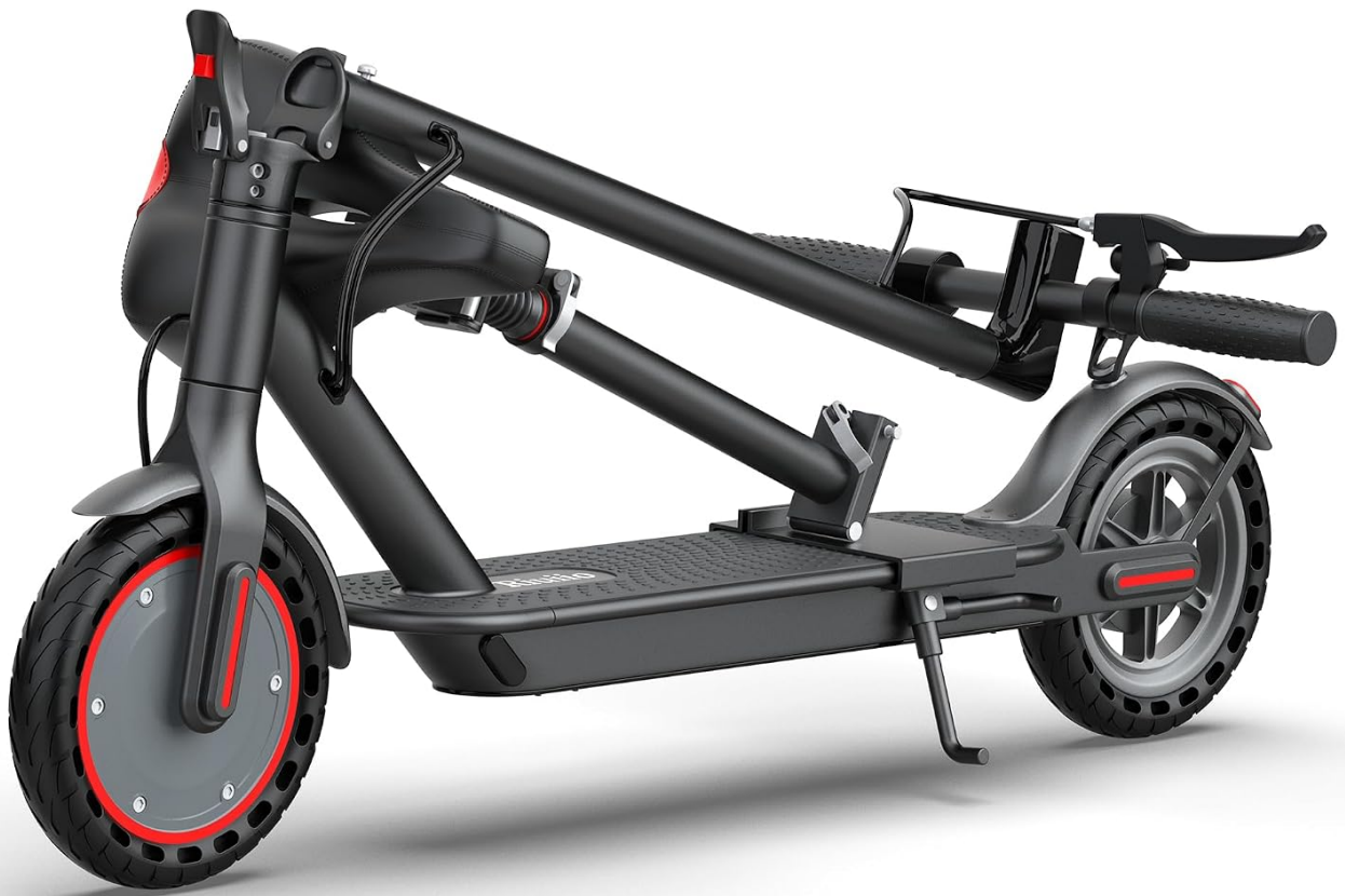
Image: Folded Electric Scooter. The scooter folds compactly for easy transport and storage.
