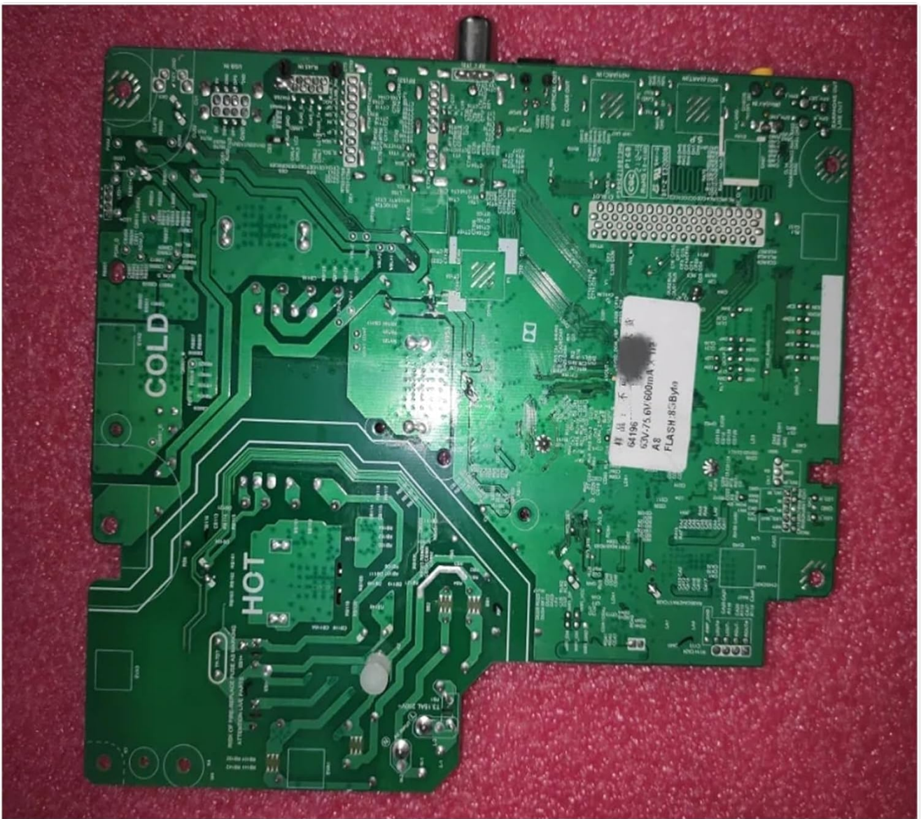
Figure 3.2: Bottom view of the TP.MT9256.PB781(T) 5mt256a TV Motherboard. This view highlights the intricate circuit traces and solder points on the reverse side of the board.
