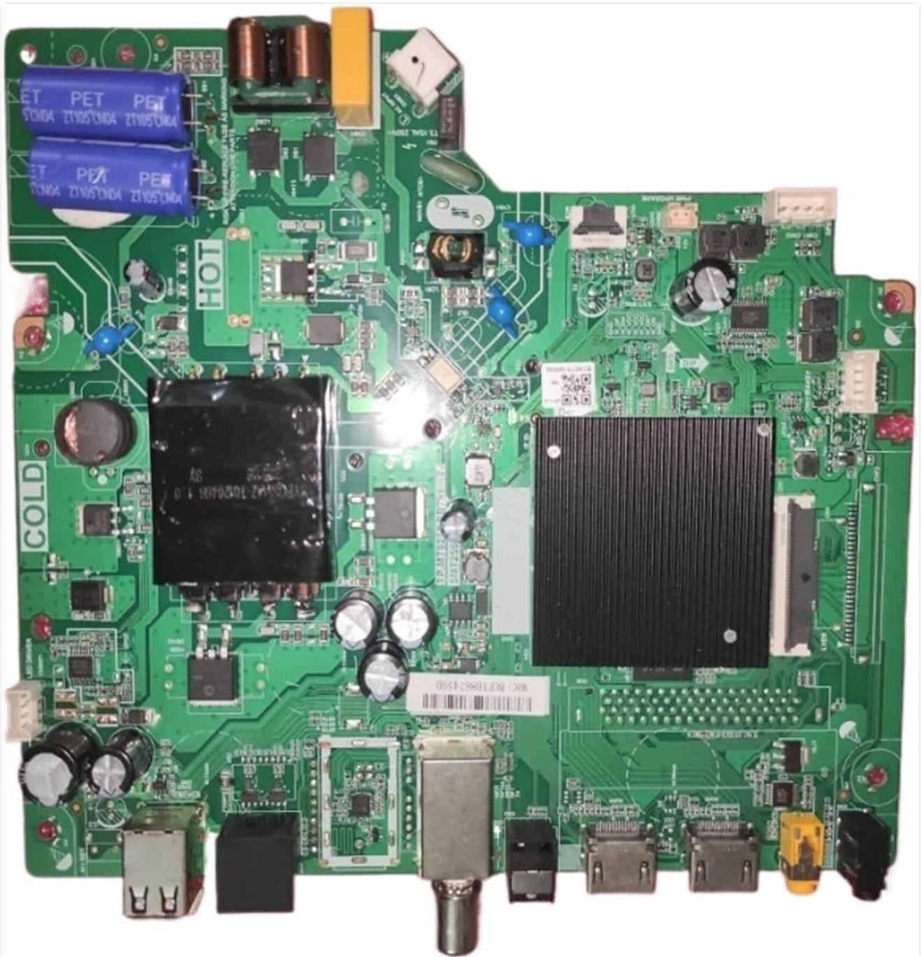
Figure 3.1: Top view of the TP.MT9256.PB781(T) 5mt256a TV Motherboard. This image displays the arrangement of major components including the main processing unit, memory modules, and various input/output ports.
