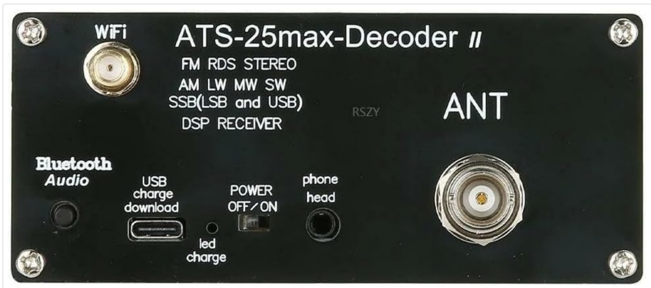
Figure 3.2: Rear view of the ATS25 Max-Decoder ii, highlighting the ANT port, WiFi port, USB charge/download port, and POWER OFF/ON switch.
