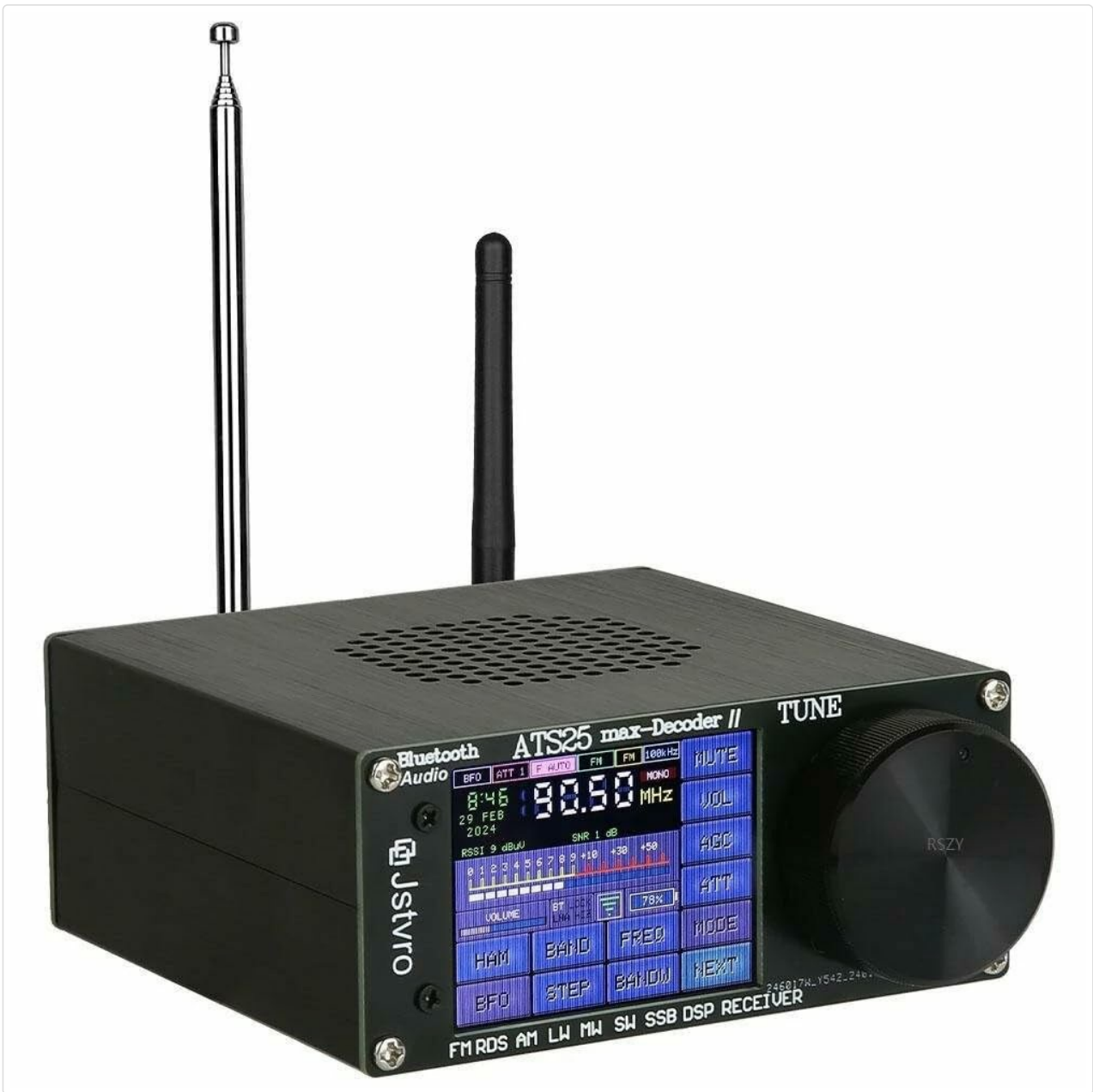
Figure 4.1: Front view of the ATS25 Max-Decoder ii, showing the touch screen interface and tuning knob.
