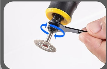
Figure 3.2: Visual guide for attaching accessories: pressing the lock button, loosening the collet nut with a wrench, inserting the accessory, and tightening the collet nut.
