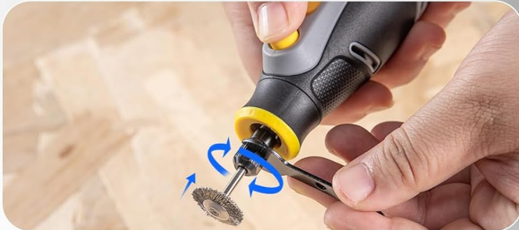
Figure 3.2: Visual guide for attaching accessories: pressing the lock button, loosening the collet nut with a wrench, inserting the accessory, and tightening the collet nut.
