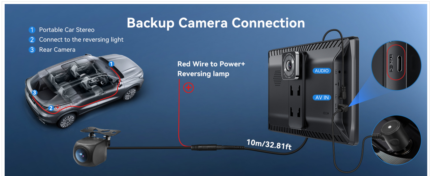
Figure 4.2: Backup Camera Connection Diagram
