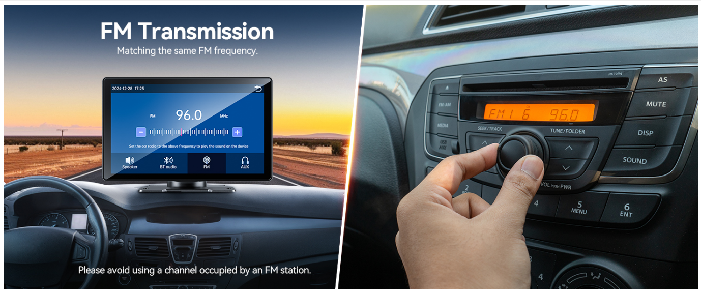
Figure 5.8: FM Transmission Setup
