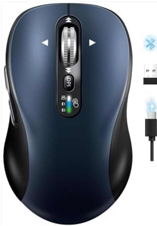
Image: Front view of the INFINMIND Wireless Multi-Device Mouse, highlighting its main buttons, scroll wheel, DPI button, and connection mode indicator lights.
