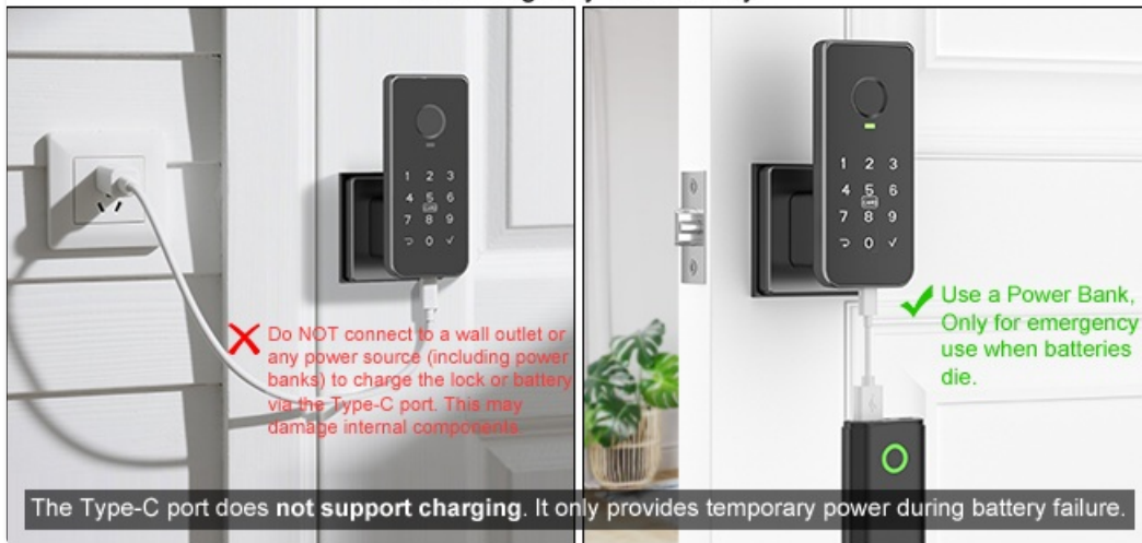
Image 5.2: Using the Type-C port for emergency power.
