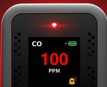
Figure 6.1: Visual and audible alerts in action, showing a high CO reading and alarm indicators.
