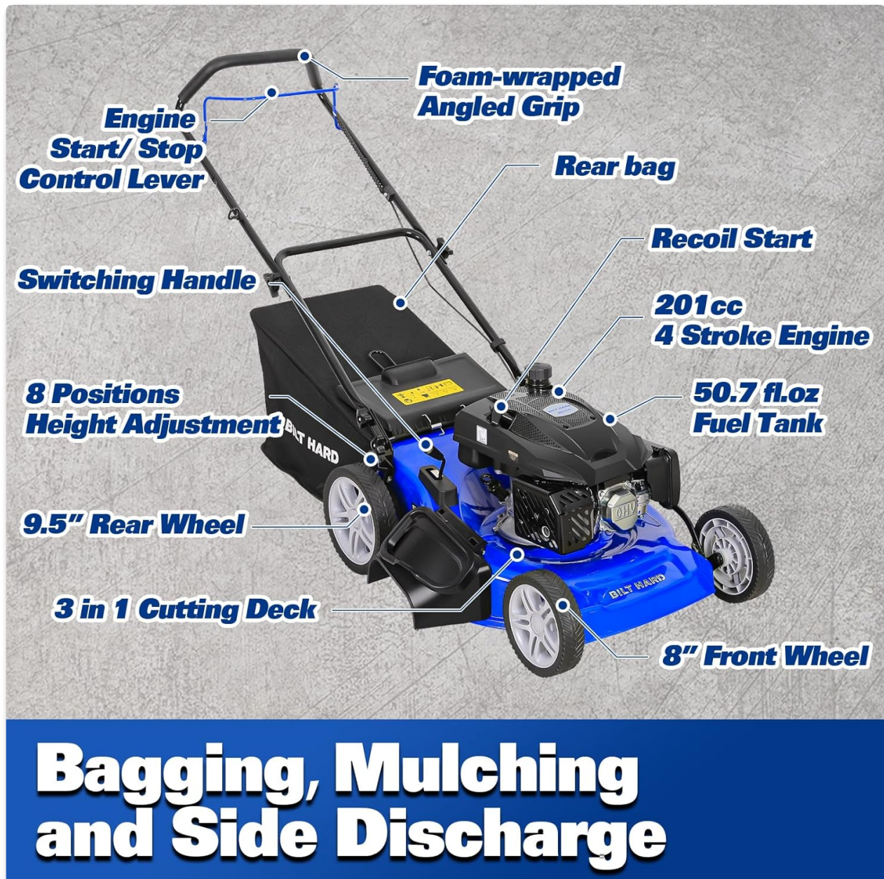
Image 3.1: Key components and controls of the lawn mower.
