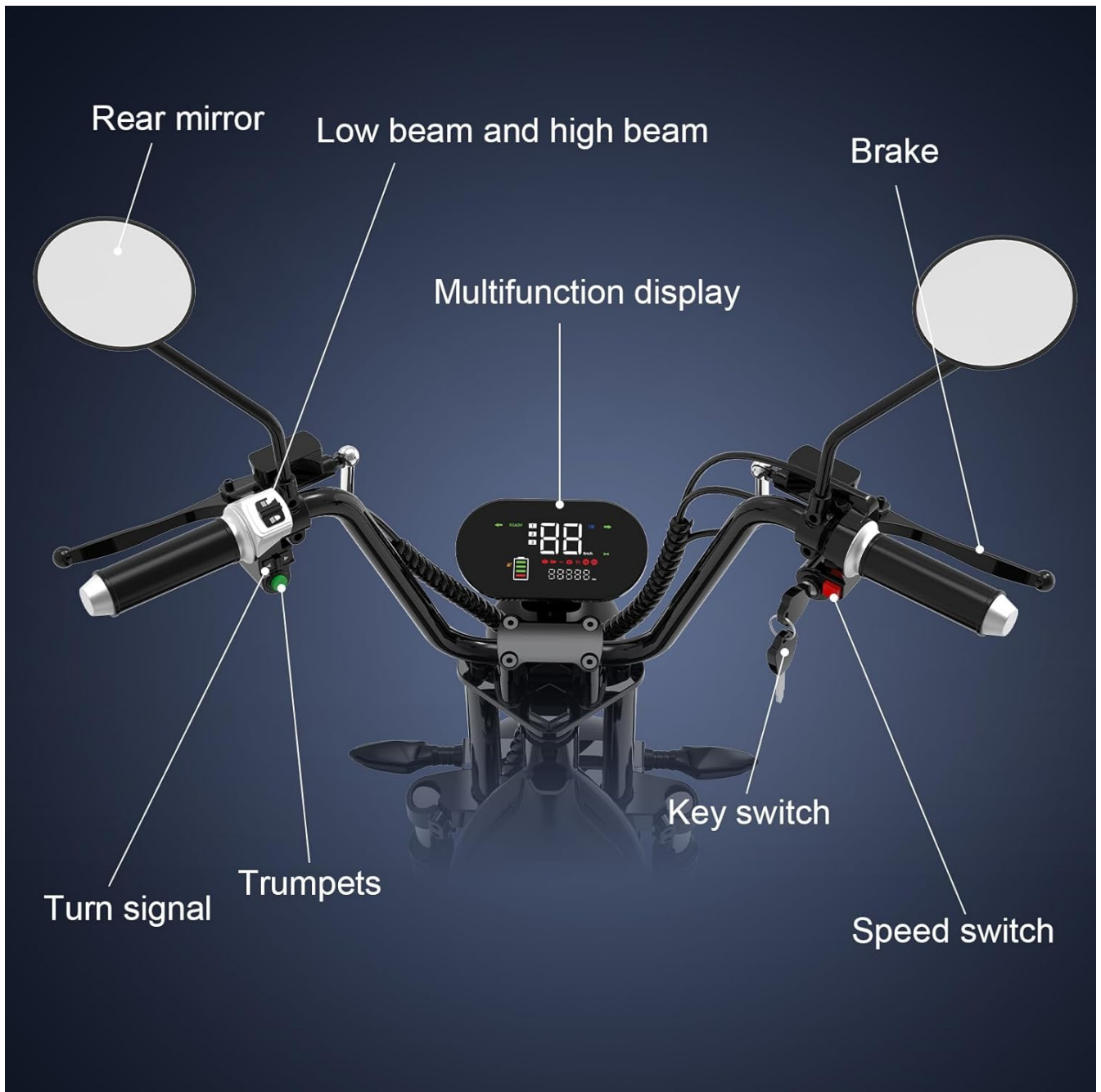
Image: An overhead view of the EVERCROSS 701 handlebars, with labels pointing to key controls: rear mirror, low beam and high beam switch, brake levers, multifunction display, key switch, speed switch, turn signal, and trumpets (horn).
