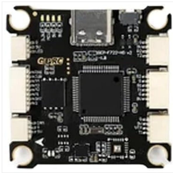
Figure 1: The F722 BLS 50A Stack, featuring the GEP-F722-HD V2 Flight Controller and the GEP-BLS50A-4IN1 ESC. This image highlights the compact design, various connection points, and the Type-C USB interface.
