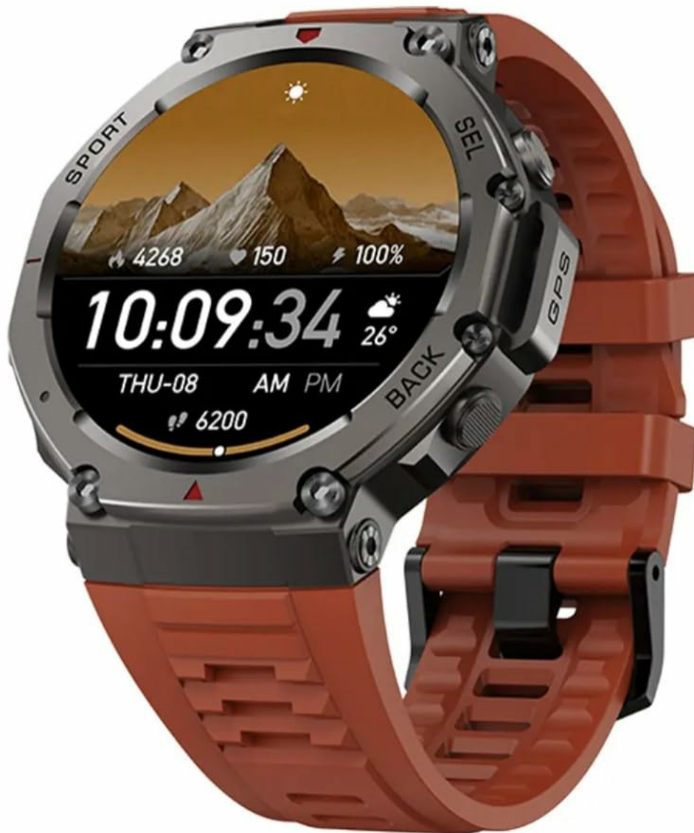
Image 4.1: Watch face showing time, date, step count, and battery level.
