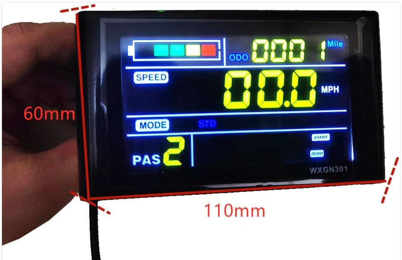
Figure 6: The WXGN301 LCD Display showing its approximate dimensions.
