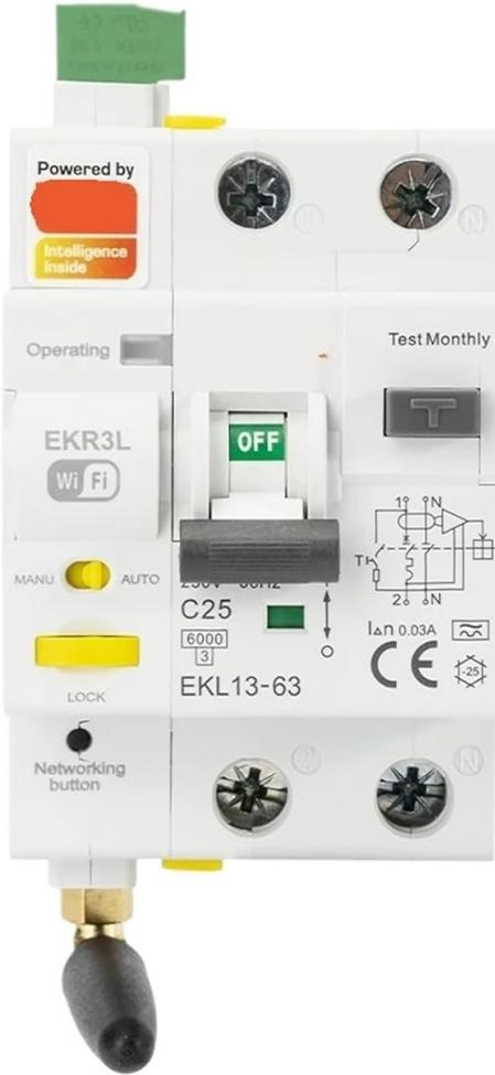
**Figure 1:** Front view of the ETEK WiFi Smart RCBO EKR3L Circuit Breaker. Key components include the main switch (OFF/ON), Test Monthly button, MANU/AUTO selector, Networking button, and WiFi indicator.
