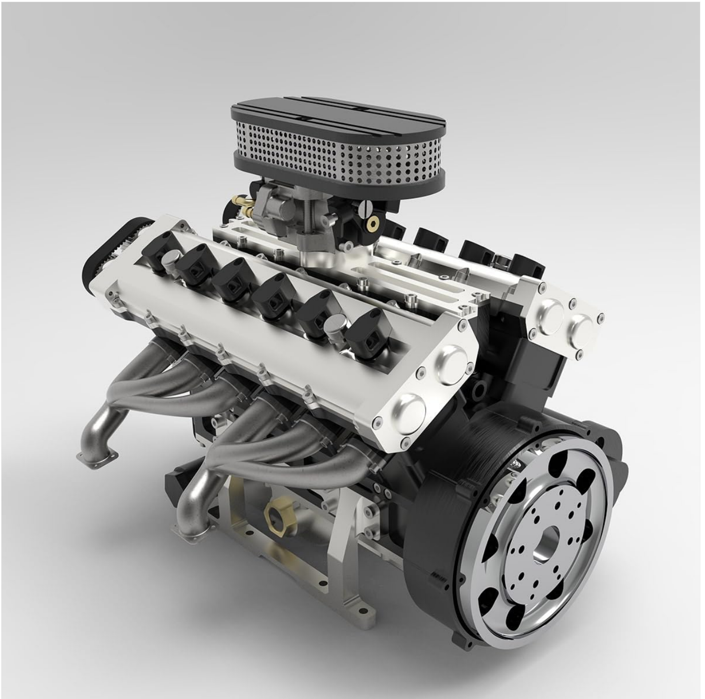
Figure 4.1: Rear-right view of the engine model, illustrating the flywheel and potential mounting points.
