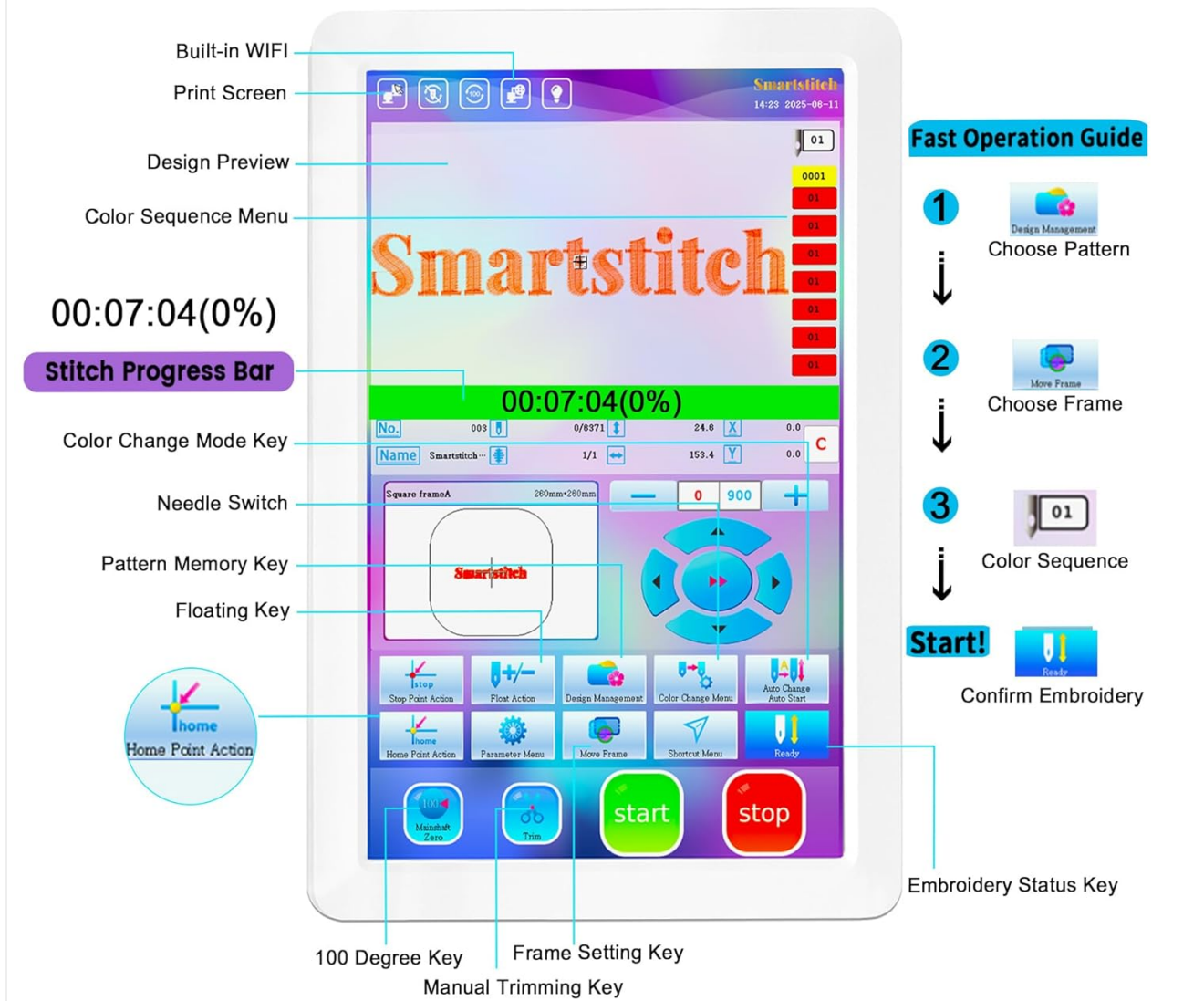
Figure 4: The 12-inch large touch screen interface, showing design preview, color sequence menu, stitch progress bar, and fast operation guide.
