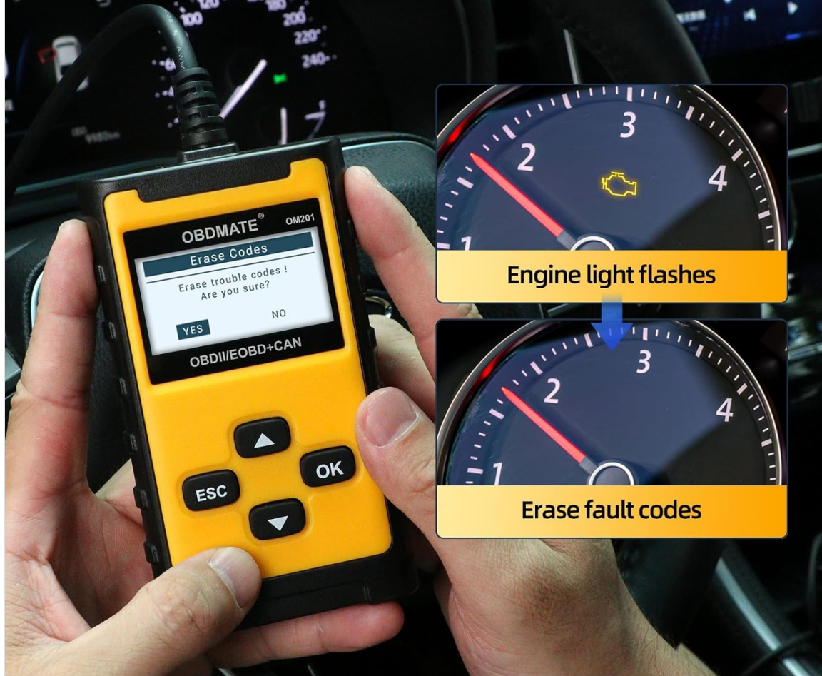
Image: The OM201 Car Scanner displaying the 'Erase Codes' prompt, asking for confirmation to clear trouble codes.
