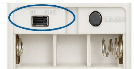
Image 4.3: The D/CFL switch located within the remote's battery compartment. This switch may need to be adjusted based on the type of light bulbs used (D for dimmable incandescent, CFL for non-dimmable LED/CFL).
