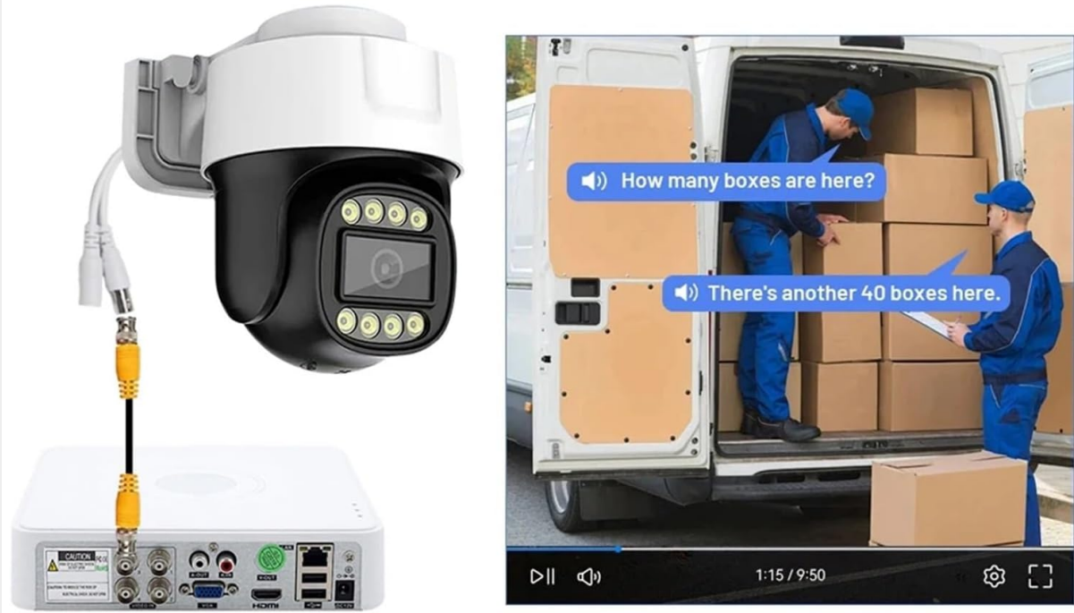
Figure 5.2: Connection diagram for TVI Coaxial Audio. The camera's built-in microphone transmits audio over the same coaxial cable as video. Connect the camera's BNC output to a DVR that supports coaxial audio functionality to obtain video with sound.
