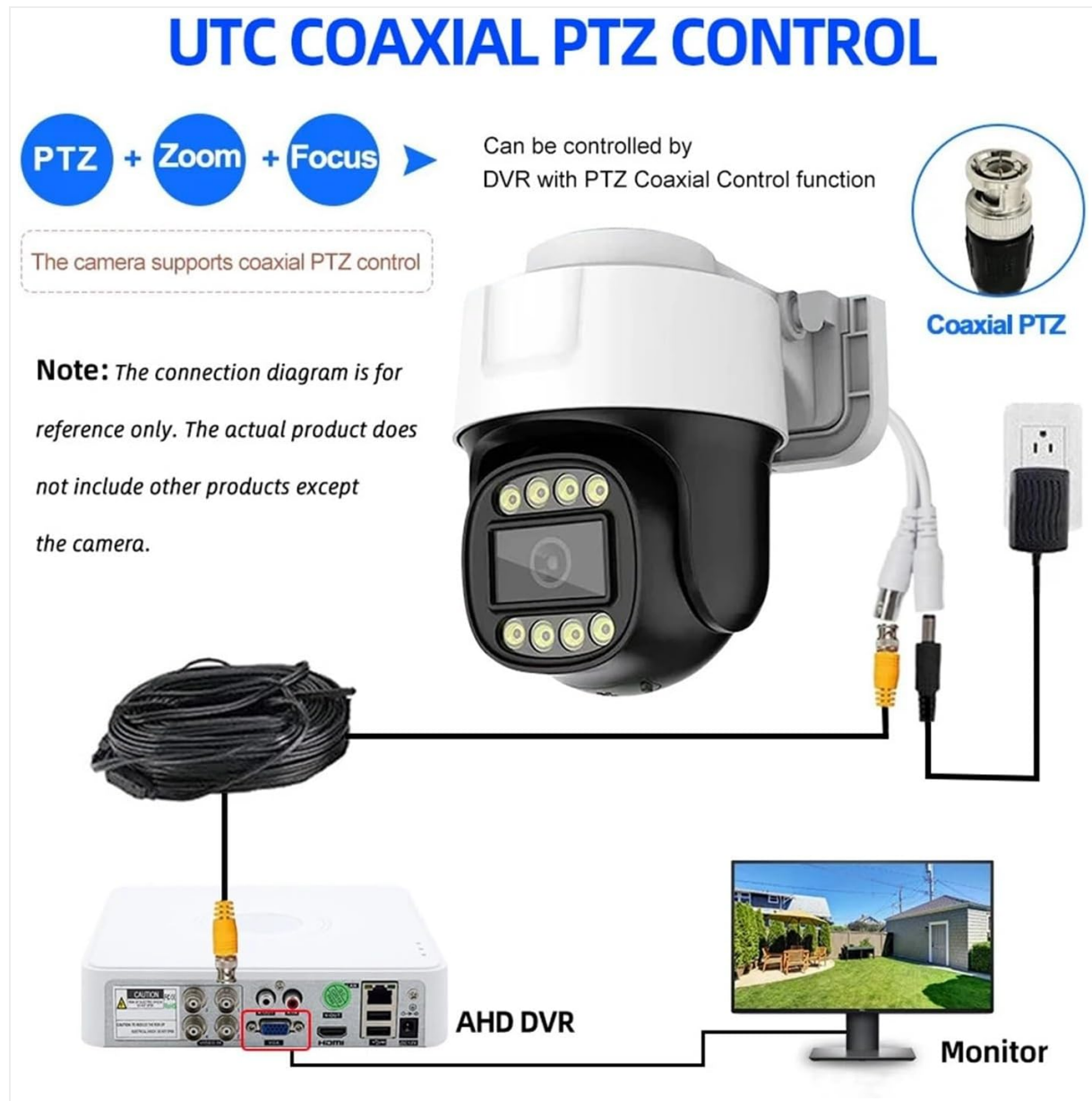
Figure 5.1: Connection diagram for UTC Coaxial PTZ Control. Connect the camera's BNC output to the AHD DVR's BNC input. Ensure the DVR supports PTZ Coaxial Control. Connect the camera to a power source.
