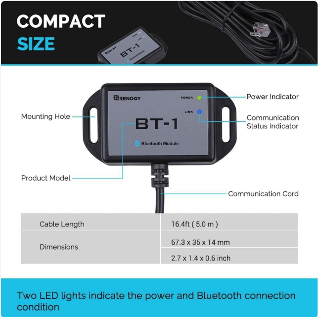
Image: A diagram of the Renogy BT-1 module showing its compact size, dimensions, cable length, and labeling its components: Power Indicator, Communication Status Indicator, Product Model, and Communication Cord.
