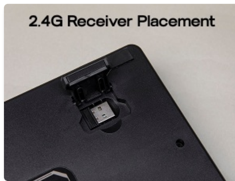
Image showing the dedicated storage slot for the 2.4G wireless receiver on the underside of the keyboard.
