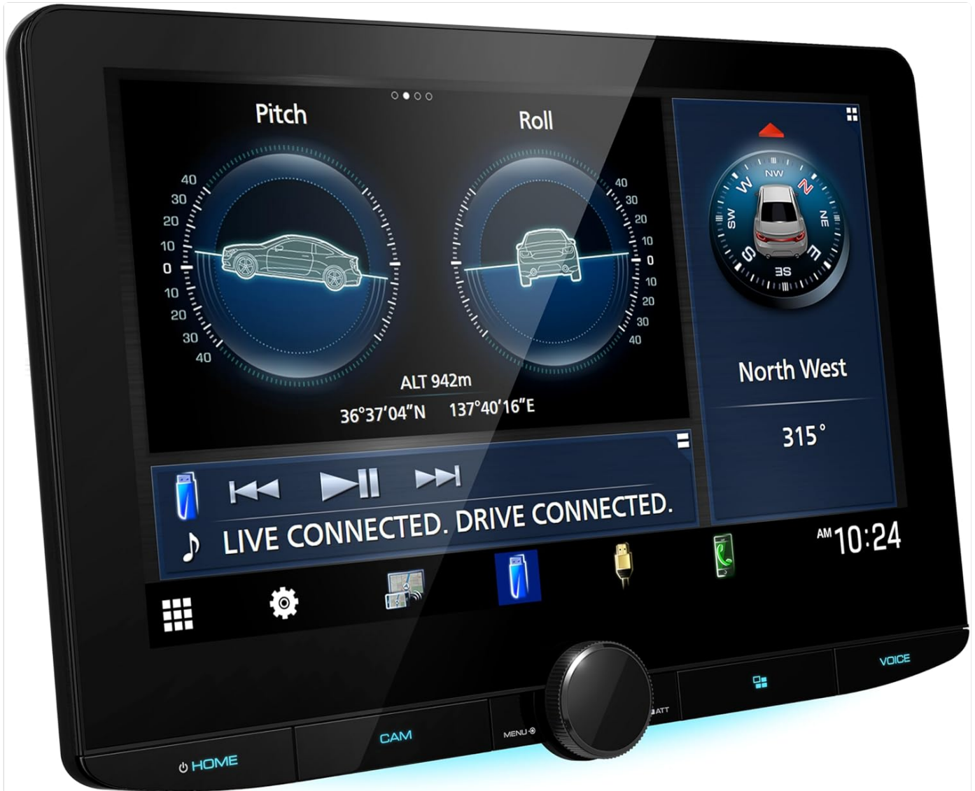
The DMX1058XR display showing vehicle pitch and roll data, accessible via iDataLink Maestro integration.
