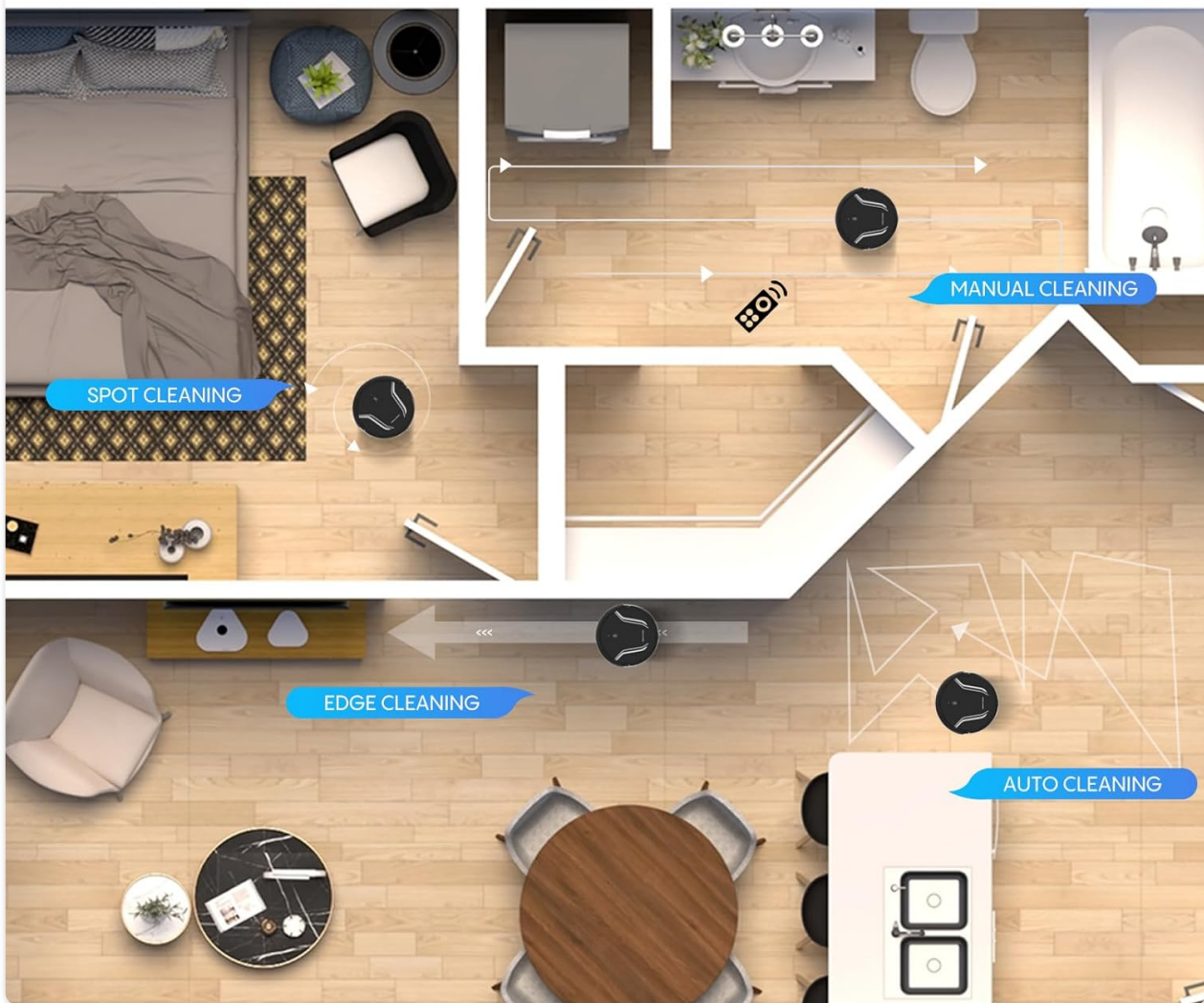
Image: An overhead diagram illustrating the four primary cleaning modes of the Bagotte A22 Robot Vacuum: Auto Cleaning, Edge Cleaning, Spot Cleaning, and Manual Cleaning, showing their typical cleaning paths within a room layout.
